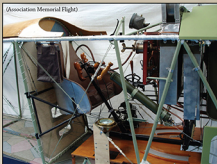
Note the linen screen (A20) behind the pilot's seat, linen wrapped around the top longerons, unpainted brass compass and aluminium rear of the seat.
