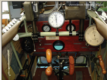
^ Instrument panel showing one arrangement of instruments. Note the tachometer in the center and altimeter (A12) on right. The bank indicator at the bottom of the panel may be correct for some aircraft but it is not an instrument that appears in the references we have for WW1 era Fokker D.VII. The twin LMG 08/15 'Spandaus' are mounted a little lower than would be expected for an airframe designed to accept the taller 185ps BMW IIIa.
