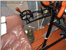
Note the throttle & mixture control (altitude compensator) levers (A20) and spark advance (A21).
