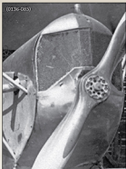
Radiator detail from very early production Jasta 28w Fokker D.VII 247/18 seen on page 18.
