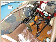
Note the control column (A16) with hand throttle (A18).
