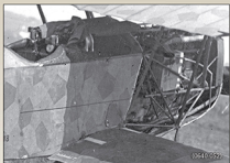
Front fuselage detail from late production Fokker built D.VII 7756/18 photographed in America. Note the late production oil tank (A6 + B2) beside the engine and 'Fokker style' triangular hatch (116) in the fuselage fabric at the wing root, both features found on late production machines.
